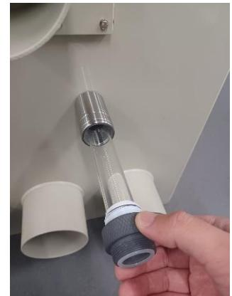
Carefully slide the Uv lamp in to the quartz sleeve and stop when only the white connection end is left.
