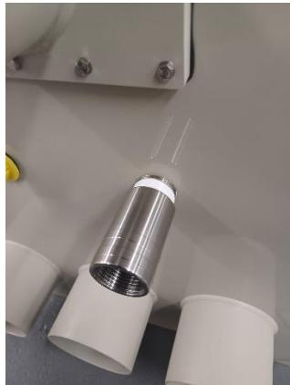
Thread with PTFE the Uv adaptor in to the per drilled UV position on your drum filter. Please note the adaptor is only needed on **BD 300, BD 300 Combi, BD 500 and BD700 models.**
